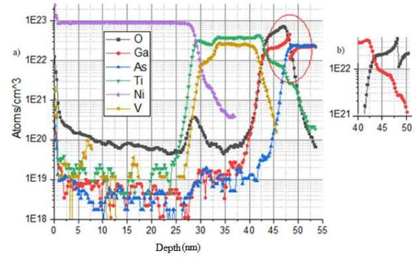
Fig. 5 SIMS studies for the  $Ga_2O_3$ -a:Ti/ $Ga_2O_3$ -a(i)/p-type GaAs (100) heterojunction
