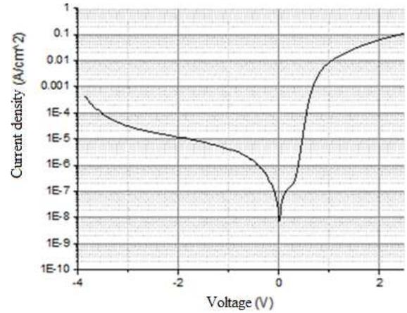
Fig. 7 J-V semi log curve for the  $Ga_2O_3$ -a:Ti/ $Ga_2O_3$ -a(i)/p-type GaAs (100) heterojunction
