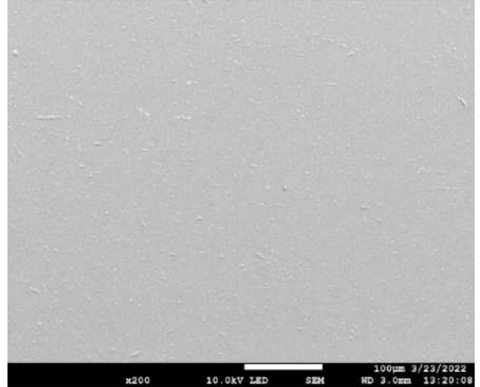
Fig. 1 SEM image for a Ga<sub>2</sub>O<sub>3</sub>-a:Ti film.
