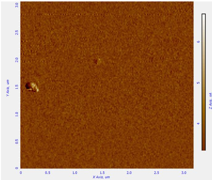
Fig. 4 AFM image for the  $Ga_2O_3$ -a:Ti/ $Ga_2O_3$ -a(i)/p-type GaAs (100) heterojunction
