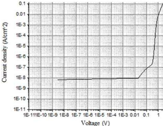
Fig. 8 J-V log curve for the  $\text{Ga}_2\text{O}_3$ -a:Ti/ $\text{Ga}_2\text{O}_3$ -a(i)/p-type GaAs (100) heterojunction
