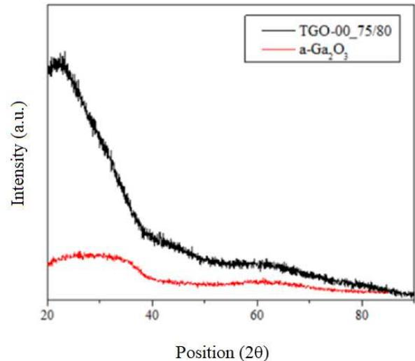
Fig. 2 XRD characterization for Ga<sub>2</sub>O<sub>3</sub>-a film
