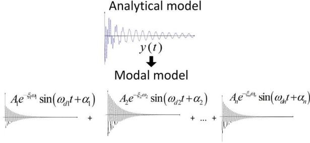
Fig. 1. Modal analysis of an electric signal
