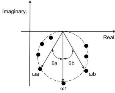
Fig. 2. Circle fit modal parameters extraction method
