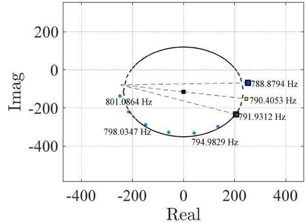
Fig. 9. Circle fit of the second resonance.
