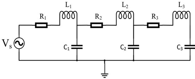
Fig. 3. Electric vibrating system.
