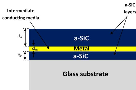
Fig.1. Cross-sectional view of the analyzed SiC/Ag/SiC multilayer structure.
