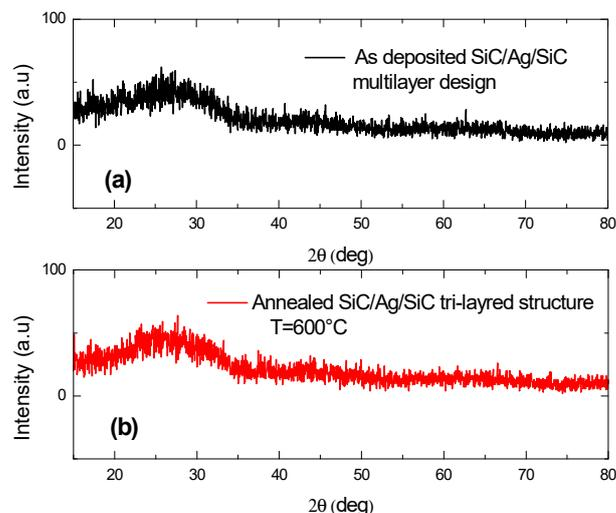
Fig. 2. X-ray diffraction patterns of the (a) sputtered SiC/Ag/SiC multilayer structure as deposited and (b) with annealing effects at 600°C.
