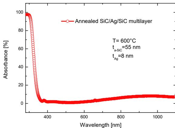
Fig. 3. Variation of the absorbance as a function of the wavelength of both prepared tri-layered structure (a) as-deposited structure. (b) annealed structure at 600°C.
