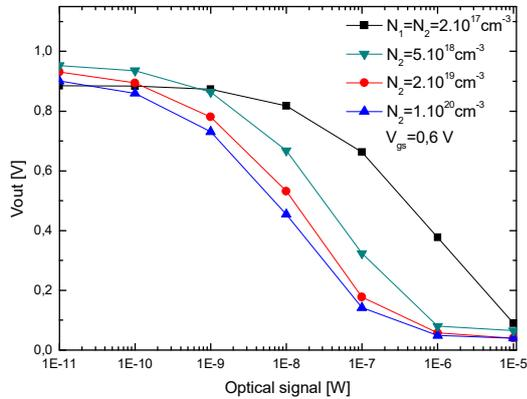
Fig. 3.  $V_{out}$  against input optical power of the investigated device for different  $N_2$  levels compared with conventional inverter with Ge-gate PT, with  $N_1=2 \times 10^{17} \text{ cm}^{-3}$ ,  $N_{ch}=2 \times 10^{17} \text{ cm}^{-3}$ ,  $V_{gs} = 0.6 \text{ V}$ .
