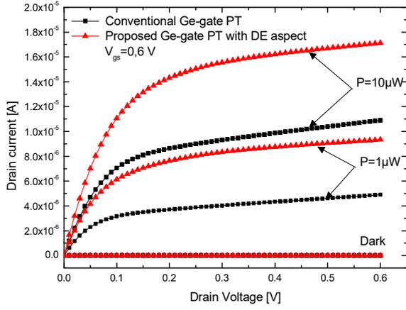
Fig. 2.  $I_{ds}$  versus  $V_{ds}$  of the proposed Ge-gate PT with DE aspect at dark and illuminated by  $1.55 \mu\text{m}$  light and power  $1 \mu\text{W}$  to  $10 \mu\text{W}$  compared with that of the conventional phototransistor with applied  $V_{gs} = 0.6$ ,  $N_1=5.10^{16} \text{ cm}^{-3}$ ,  $N_2=5.10^{18} \text{ cm}^{-3}$ .
