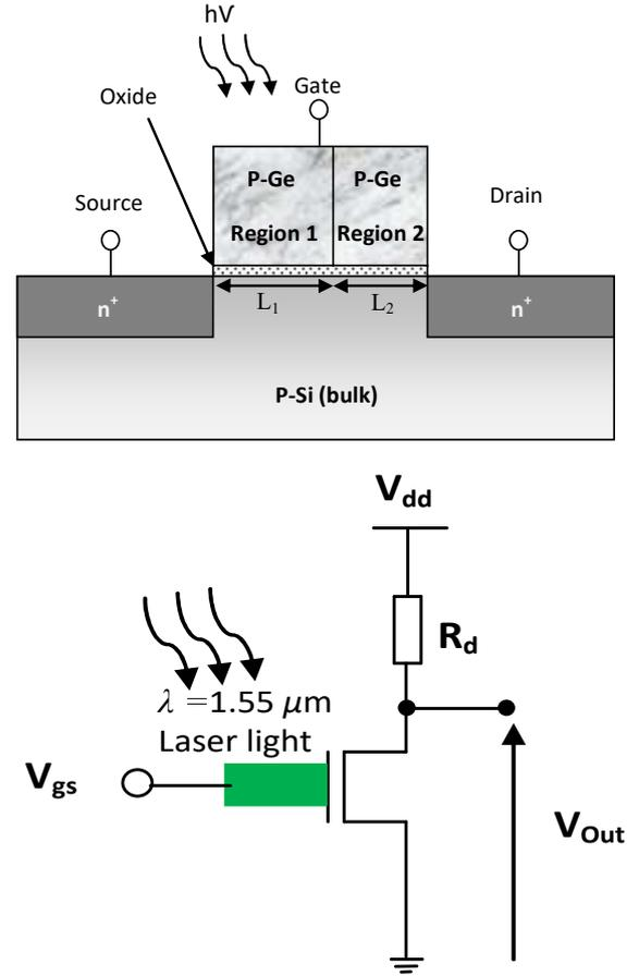
Fig.1. (a) Cross-sectional view of the proposed Ge-gate phototransistor based on DE aradigm. (b) Investigated optical inverter circuit based on the proposed Ge-gate PT device with DE aspect on MOSFET platform
