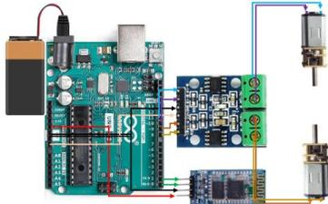
Fig. 2. Schematic of the Developed CPM device. (HSI-CPM)
