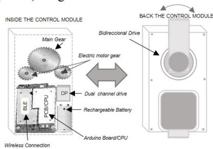
Fig. 3. Mechanical and Electric System Design
