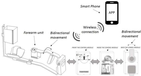
Fig. 7. HS1-CPM device with Mobile application and Arduino
