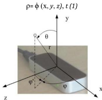
Fig. 8. The cartesian and spherical coordinate systems used to describe positions in the controller's sensory space.
