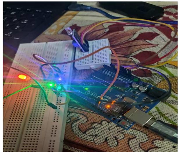
Figure 3: Practical Implementation of Optical transducer and Arduino UNO
