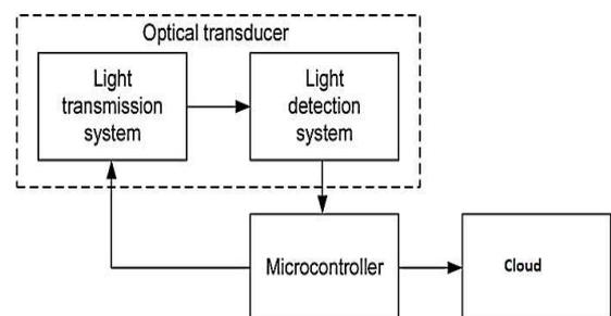
Figure 1:Block Diagram of Optical Transducer connected to Microcontroller[4]
