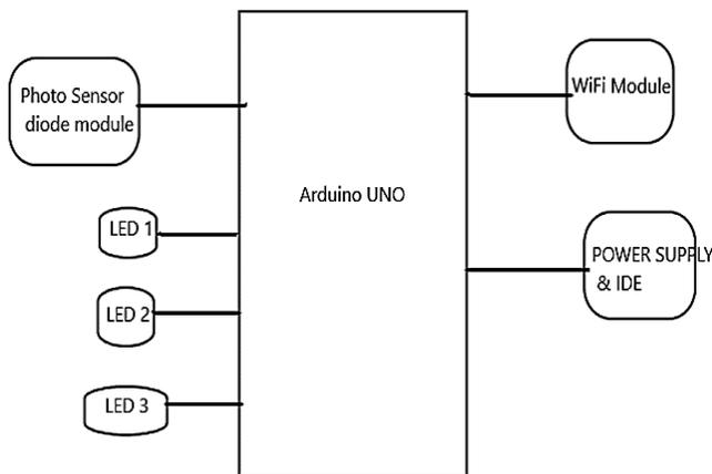
Figure 2: Arduino UNO with connected components
