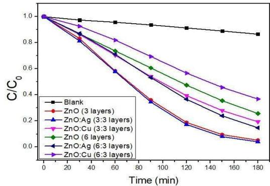
Fig. 5. Photocatalytic decoloration rate of ZnO thin films.
