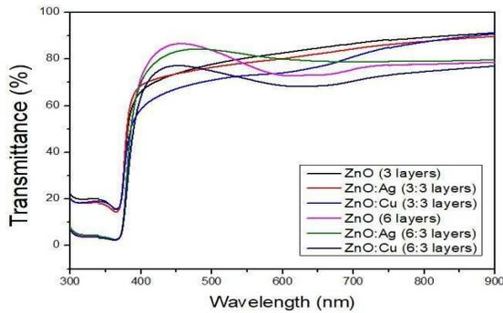
Fig. 3. Optical transmission spectrum of ZnO thin films.
