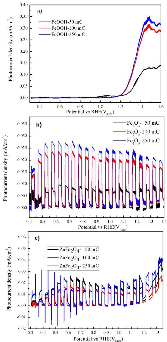
**Fig. 4.** Photocurrent of a) FeOOH, b)  $\alpha$ - $Fe_2O_3$ , and c)  $ZnFe_2O_4$  thin films deposited.
