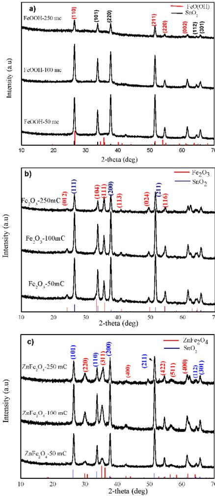
**Fig. 1.** XRD spectra of a) FeOOH, b)  $\alpha$ -Fe<sub>2</sub>O<sub>3</sub>, and c) ZnFe<sub>2</sub>O<sub>4</sub> thin films deposited
