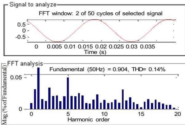
Fig.4.1. Terminal voltage at PCC along with harmonics spectrum
