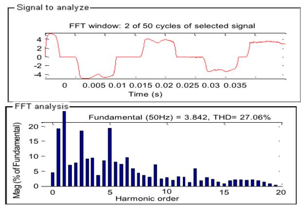
Fig. 4.3 Terminal and load current with harmonic spectrum
