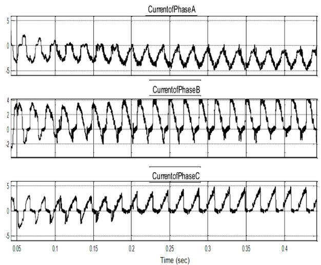
Fig 3.4 Non-linear load current of Phase A, B and Phase C
