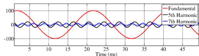
Fig 2.4. Waveform representation of different harmonics
