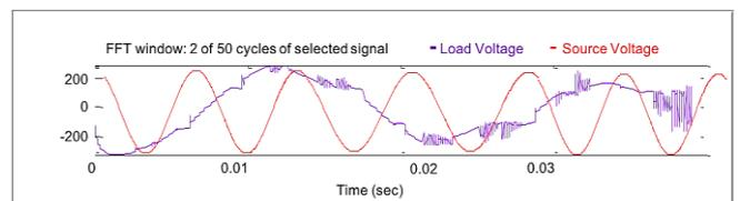
Fig.3.5. Non-linear load voltage and source voltage
