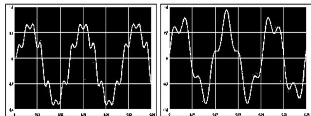
Fig 2.3. Waveform-shape difference between harmonics and inter harmonics
