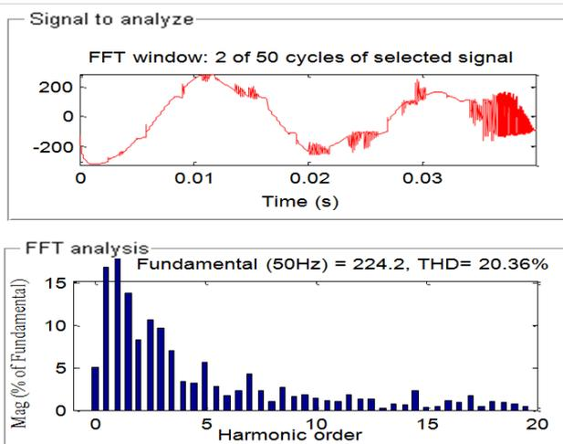
Fig. 4.2 Load voltage (VL) at PCC along with harmonics spectrum
