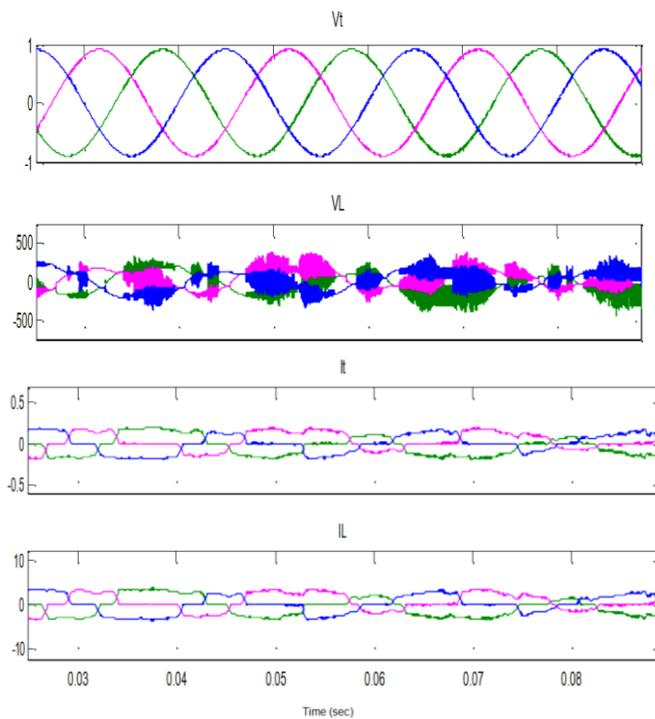
Fig. 3.2. Terminal voltage ( $V_t$ ), load voltage ( $V_L$ ), terminal current ( $I_t$ ) and load current ( $I_L$ ) performance
