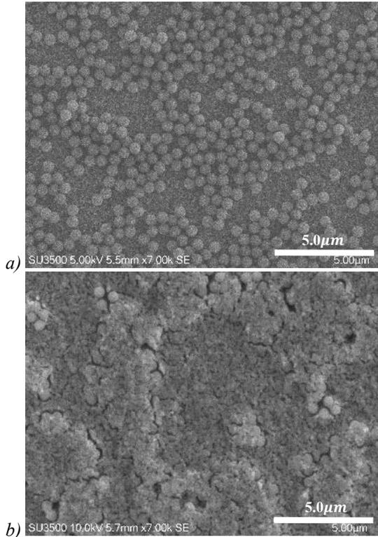
**Figure 3.** SEM images of NPs bilayer configurations: a) Titania-Silica NPs configuration: the bottom layer is made with titania NPs with 1:2 concentration deposited at 4000 rpm and the top NPs layer is made with silica NPs with a concentration of 1500 rpm, and b) is the Silica-Titania NPs configuration, it is made with the same parameters than another configuration.
