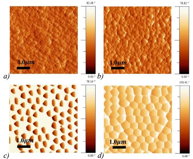
**Figure 4.** Phase contrast images of NPs monolayer NPs before and after annealing process: a) Titania NPs without thermal treatment, b) Titania NPs thermally annealed at 1100 °C for 30 minutes, c) Silica NPs before thermal treatment and d) Silica NPs thermally annealed at 1100 °C for 30 minutes.
