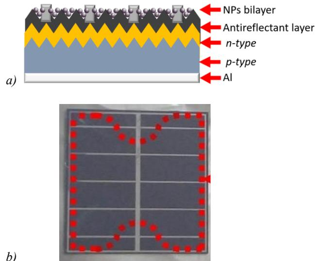
**Figure 2.** a) Basic structure of a c-Si solar cell and b) NPs deposited inside the red dashed line on the c-Si solar cell of 1×1 cm dimension.
