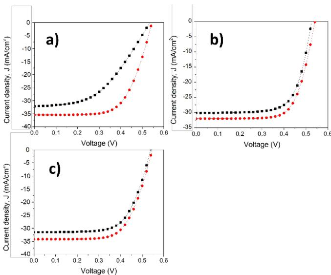
Figure 7. Current density vs Voltage curves of solar cells: before annealing process/without NPs configuration (black line) and with Titania-Silica NPs configuration/thermal treatment (red line). Thermal treatment at 400°C: a) 10 min, b) 20 min and at 500°C: c) 30 min.
