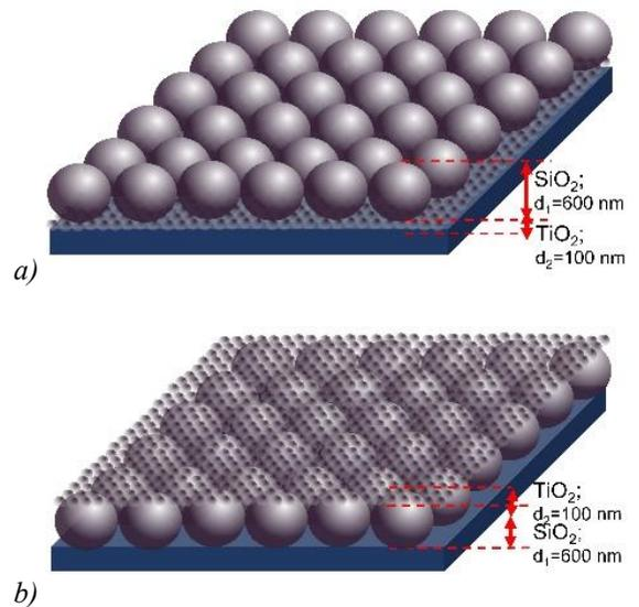
**Figure 1.** Schematics of nanoparticles (NPs) arrays: a) Titania-Silica NPs configuration and b) Silica-Titania NPs configuration.
