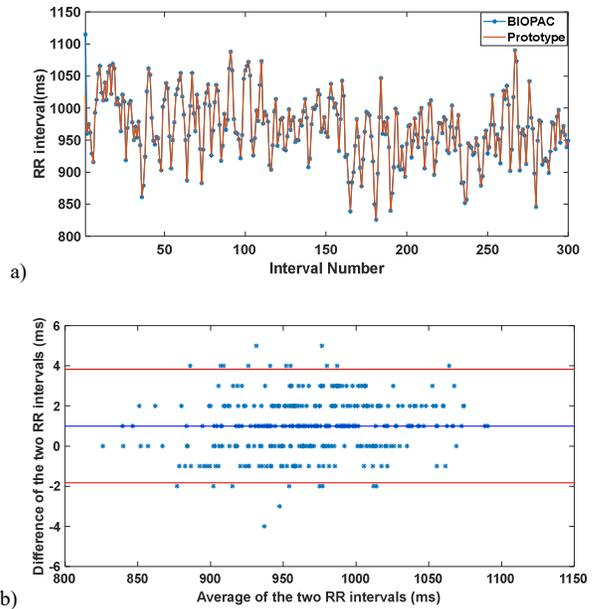
Fig. 8. Validation of the performance of the designed monitor. a). Tachogram b). Bland-Altman plot
