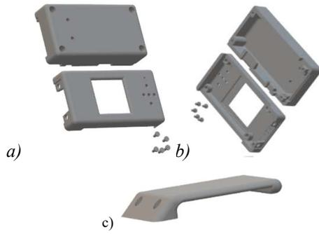
Fig. 5. Monitor case design. a) Upper face. b) Lower face. c) Fastening tab.
