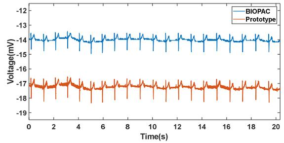
Fig. 7. Comparison of the records taken by the BIOPAC and the monitor at a sampling frequency of 1000 Hz and without input filters.
