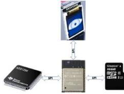
Fig. 1. Main components of the long-term continuous ambulatory ECG monitor of 3 leads with R wave detection in real time.
