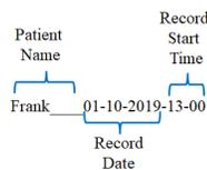
Fig. 3. Format of the name of the directory where the logs are stored.
