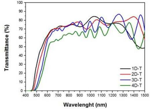
Figure 2: Transmittance of Cu<sub>2</sub>O thin films deposited
