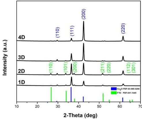
Figure 1: XRD spectra of Cu<sub>2</sub>O thin films deposited
