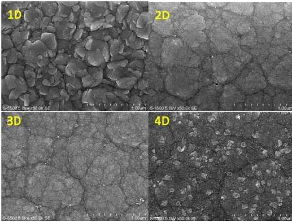
Figure 4: FE-SEM images of  $\text{Cu}_2\text{O}$  thin films deposited
