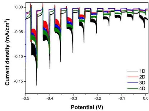
Figure 7: Photocurrent of  $\text{Cu}_2\text{O}$  thin films deposited
