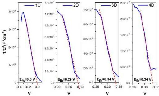
Figure 5: Flat band potential of  $\text{Cu}_2\text{O}$  thin films deposited
