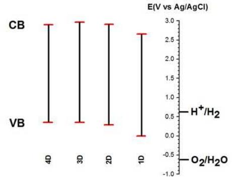
Figure 6: Band alignment of  $\text{Cu}_2\text{O}$  thin films for hydrogen production
