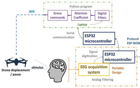
Fig. 1. Diagram of neurofeedback system developed
