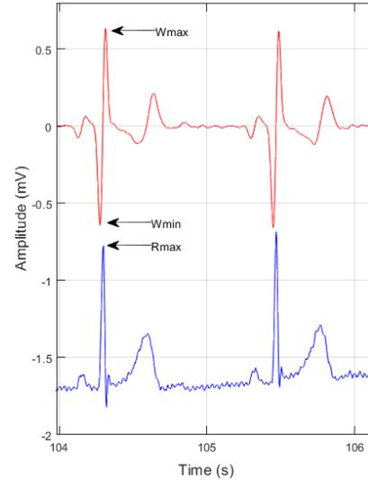
Fig. 2. ECG (bottom) and its CWT at scale 3 (top) for R-peak detection (Rmax).
