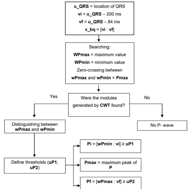
Fig. 6. Flowchart for P wave onset (Pi), P wave peak (Pmax) and P wave end (Pf) delineation.
