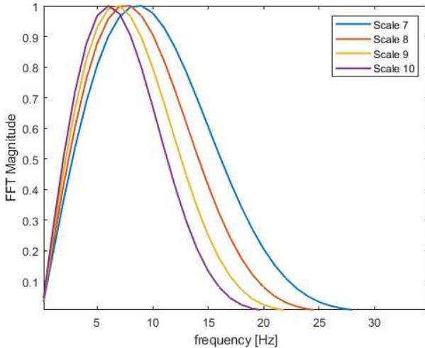
Fig. 1. Equivalent filter bandwidths at a sampling frequency,  $f_s = 250$  Hz.
