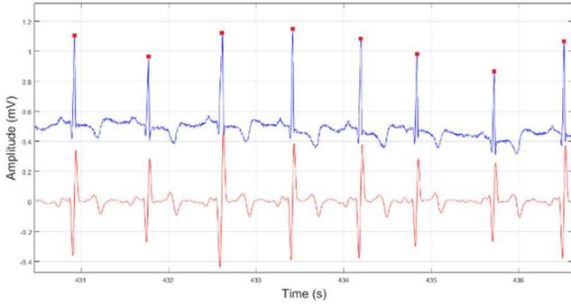
Fig. 7. ECG (top) with type of complex qRs from sel100 record and CWT (bottom) at scale 3.
