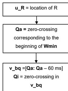
Fig. 5. Flowchart for Q onset (Qi) and Q peak (Qa) delineation.
