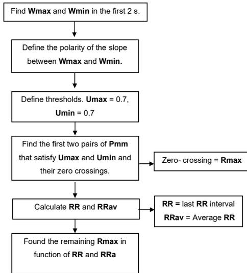
Fig. 3. Flowchart for R wave peak (Rmax) detection.
