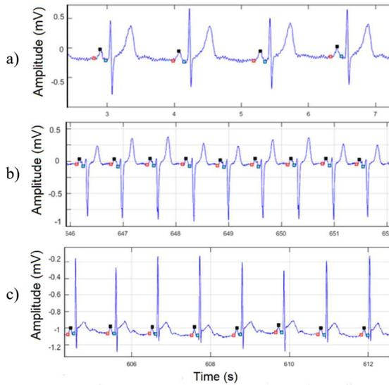
Fig.9. Segments of ECG recordings from the QT database with detections of the P-wave onset, peak and end. a). Record sel117. b). Record sel302. c). Record sel0104.
