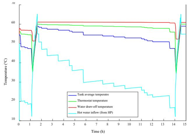
Fig. 6. Hot water draw-off, inflow, tank average, and thermostat temperature variation in the storage tank.
