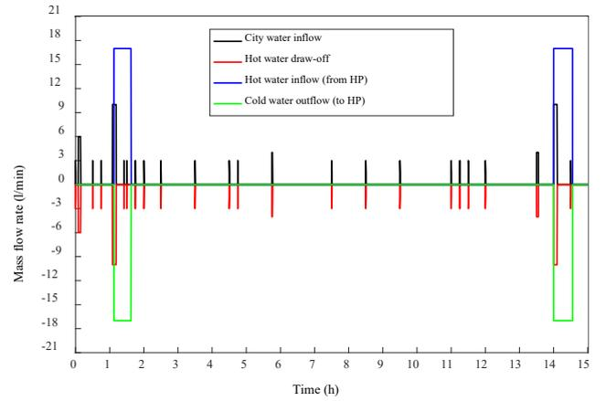
Fig. 3. Inflow and outflow profile for the storage tank.
