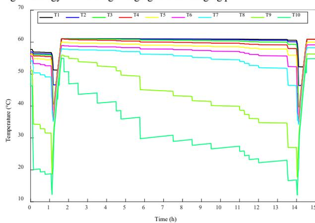
Fig. 5. Temperature distribution in the water storage tank.
