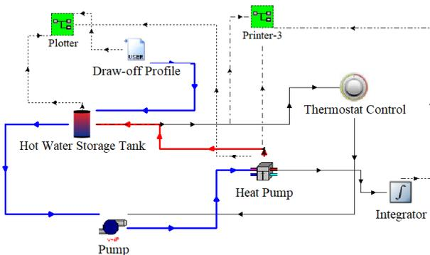
Fig. 2. Schematic of a HPWH system modeled in TRNSYS.
