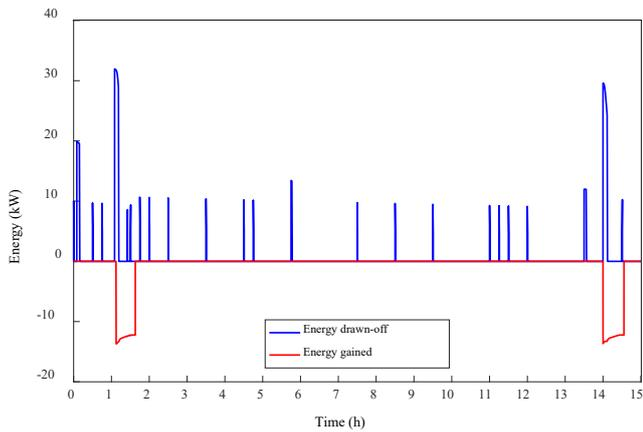
Fig. 4. Energy flow during charging and discharging processes.
