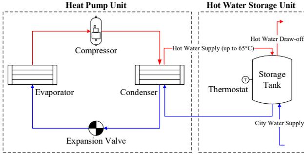
Fig. 1. Schematic of the HPWH cycle.
