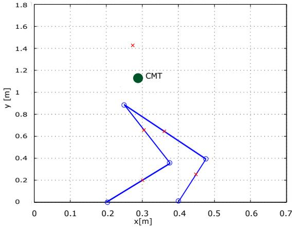
Figure 4: Center of mass of the 4 DOF model
