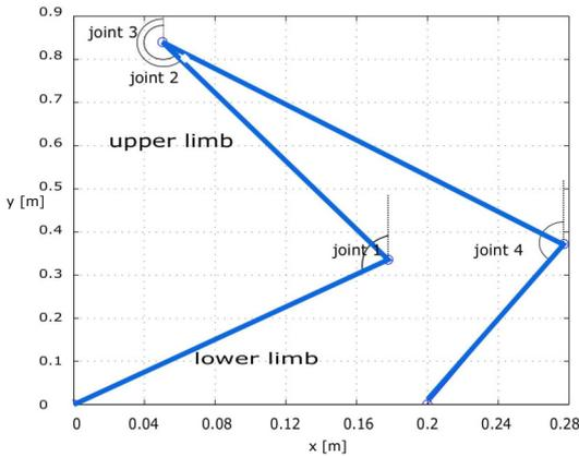
Figure 1: 4 DOF model for walking analysis
