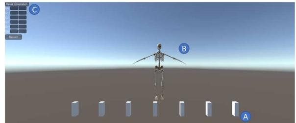
Fig. 3. User interface of the proposed developed IMU-based Mocap system. A) Boxes indicating IMU orientations. B) Skeleton avatar that moves its joints in real time. C) User interaction controls.
