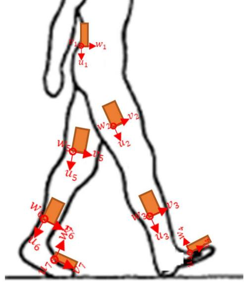
Fig.1. The orange color boxes indicate the Xsens MTx IMU sensor placement. While red arrows indicate the sensor vector orientations, and sensor number.
