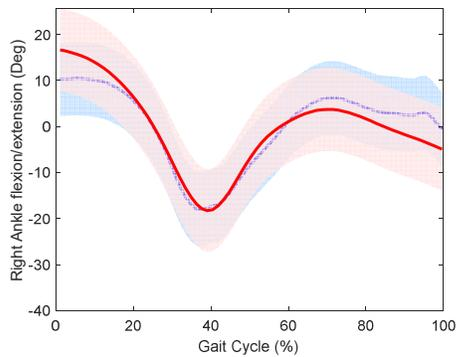
Fig. 10. Right Ankle flexion/extension joint kinematics. In blue color kinematics obtained with Vicon. In red color kinematics obtained with the proposed system. The shaded areas represent 1 mean standard deviation of the signals. RMSE=2.97 DEG.
