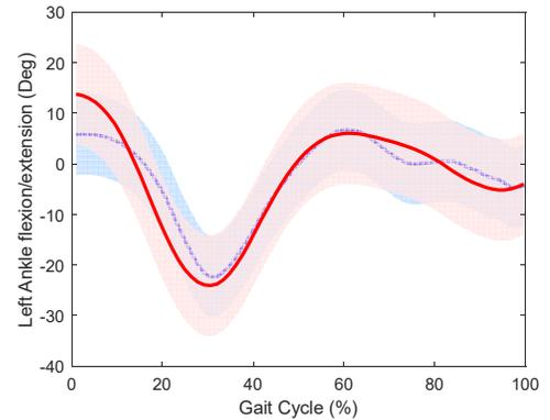
Fig. 9. Left Ankle flexion/extension joint kinematics. In blue color kinematics obtained with Vicon. In red color kinematics obtained with the proposed system. The shaded areas represent 1 mean standard deviation of the signals. RMSE=3.26 DEG.
