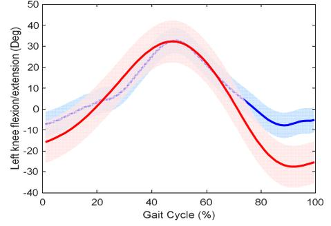
Fig. 7. Left Knee flexion/extension joint kinematics. In blue color kinematics obtained with Vicon. In red color kinematics obtained with the proposed system. The shaded areas represent 1 mean standard deviation of the signals. RMSE=9.9 DEG.
