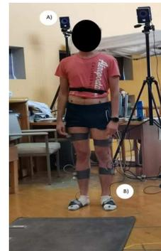
Fig. 4. Test setup. A) Vicon system cameras placed around the measurement area. B) Test subject with reflective markers and inertial sensors placed over him.
