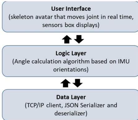
Fig. 2. Software Layer Architecture. The first layer corresponds to the user interface. The second layers calculates the joint angles based on IMU vector orientations. The third layer corresponds to the data
