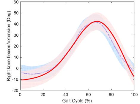
Fig. 8. Right Knee flexion/extension joint kinematics. In blue color kinematics obtained with Vicon. In red color kinematics obtained with the proposed system. The shaded areas represent 1 mean standard deviation of the signals. RMSE=3.42 DEG.
