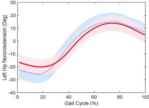
Fig. 5. Left Hip flexion/extension joint kinematics. In blue color kinematics obtained with Vicon. In red color kinematics obtained with the proposed system. The shaded areas represent 1 mean standard deviation of the signals. RMSE=4.58 DEG.
