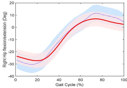
Fig. 6. Right Hip flexion/extension joint kinematics. In blue color kinematics obtained with Vicon. In red color kinematics obtained with the proposed system. The shaded areas represent 1 mean standard deviation of the signals. RMSE=2.96 DEG.
