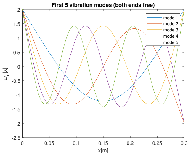
Fig. 3. Vibrations mode-shapes of a uniform beam.
