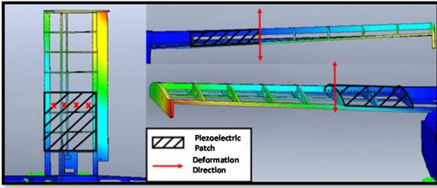
Fig. 6 First proposal for piezoelectric patch positioning on wing
