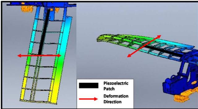
Fig. 7 Second proposal for piezoelectric patch positioning on wing
