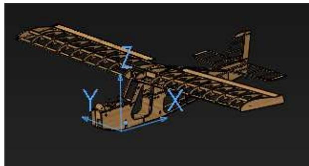
Fig. 1 Aircraft coordinate system
