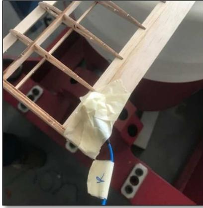
Fig. 2. Mounting Accelerometer
