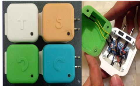
Fig. 3. Command Tokens designed with an electronic identification system requiring an electromechanical connection.
