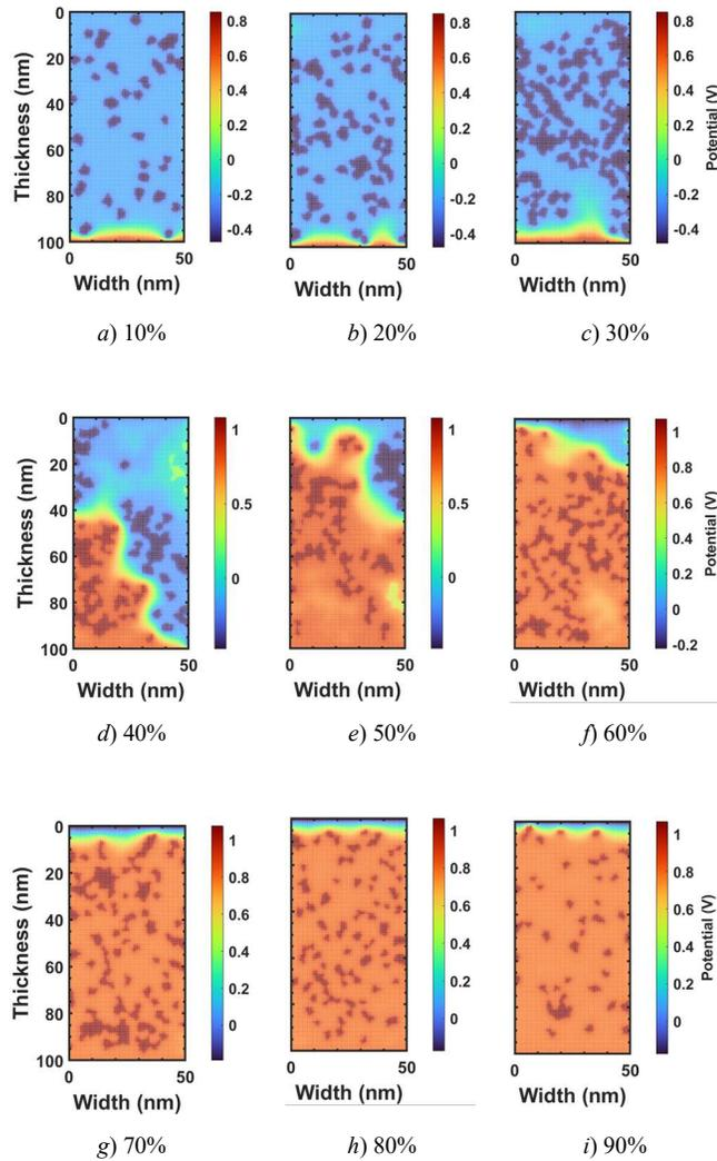
Fig. 3. Electric potential for morphology with different percentage of acceptor material under short circuit condition and  $\mu_D = \mu_A$ . The red and the blue colors represent the maximum and the minimum, respectively.
