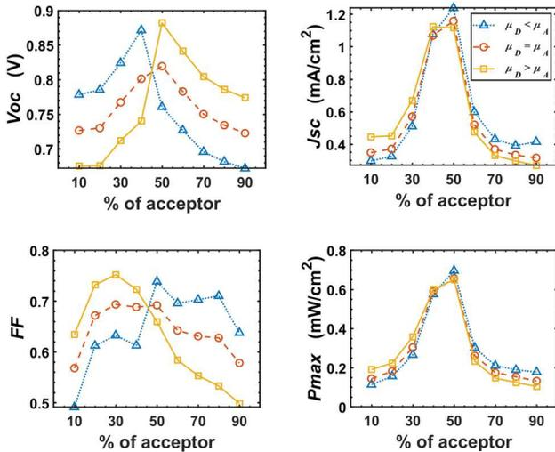
Fig. 6. Electrical parameters of the OSCs with different mobilities as a function of percentage of acceptor material.
