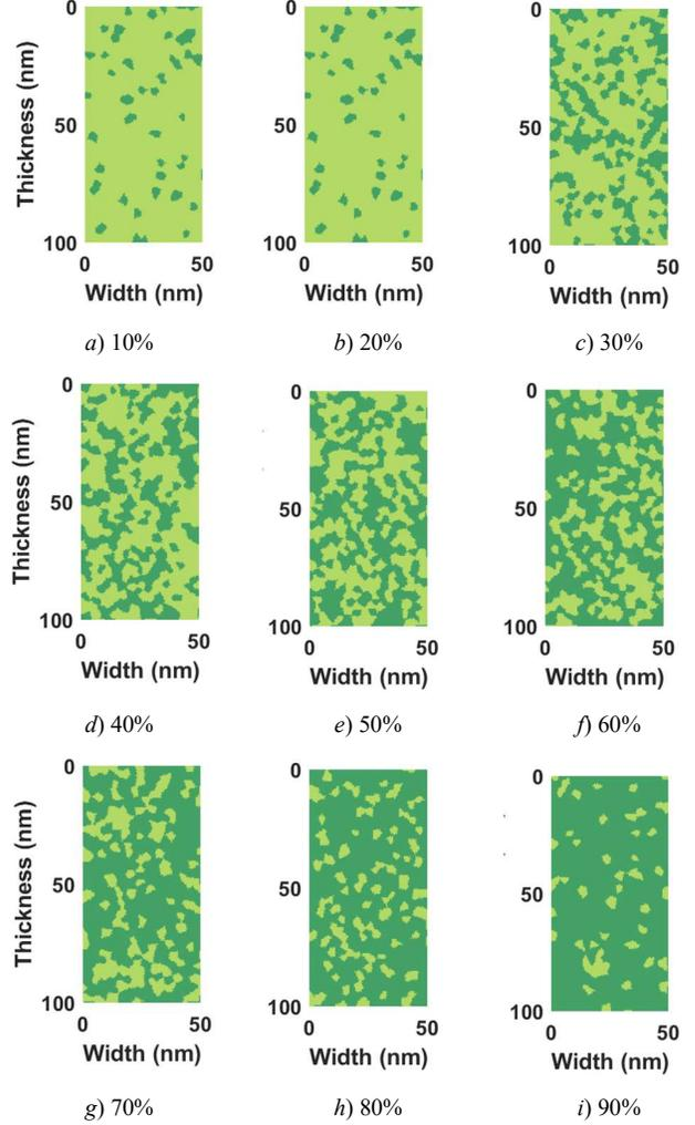
Fig. 2. Morphologies of the active layer with different percentage of acceptor material. Dark green areas correspond to acceptor phases and light green to donor phases.
