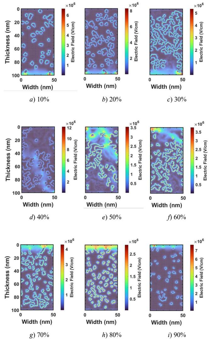
Fig. 4. Electric field for morphology with different percentage of acceptor material under short circuit condition and  $\mu_D = \mu_A$ . The red and the blue colors represent the maximum and the minimum, respectively.
