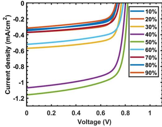
Fig. 5. Current density–voltage characteristics of bulk heterojunction solar cells with different percentage of acceptor material.
