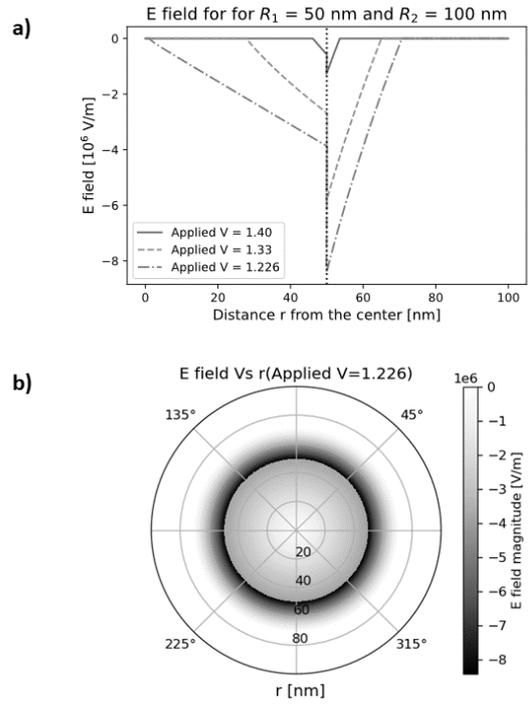
Fig. 6. a) Electric field in radial terms for the P-N Heterojunction b) Top view of  $E$  in the P-N Heterojunction.
