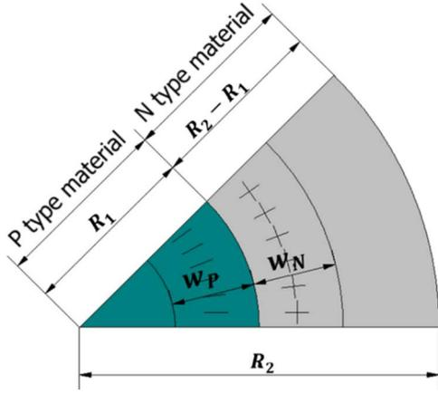
Fig. 2. Schematics of the P-N radial nanowire heterojunction dimensions.
