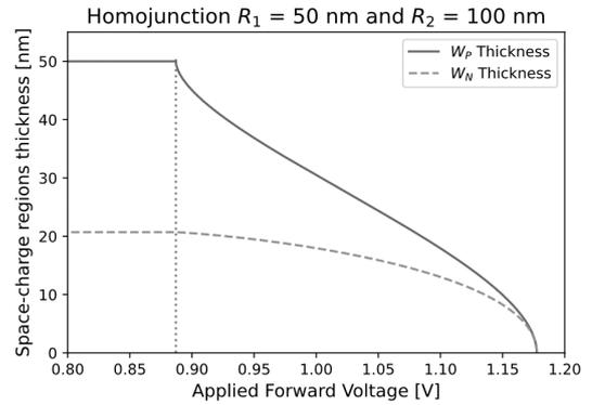
Fig. 10. Space charge thickness  $w_N$  and  $w_P$  for the symmetric InP P-N homojunction.
