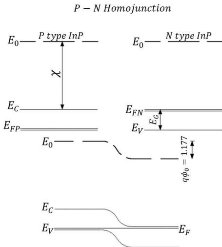
Fig. 9. InP homojunction band diagram.
