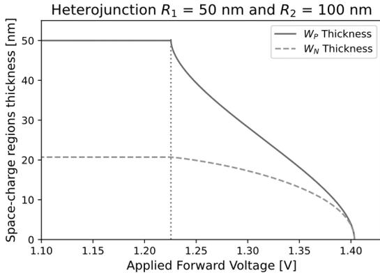
Fig. 5. Space charge thickness  $w_N$  and  $w_P$  for the Si(P)/InP(N) nanowire heterojunction diode.
