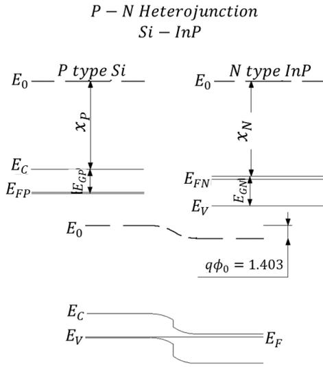
Fig. 4. Band diagram of the P-N Si/InP device.
