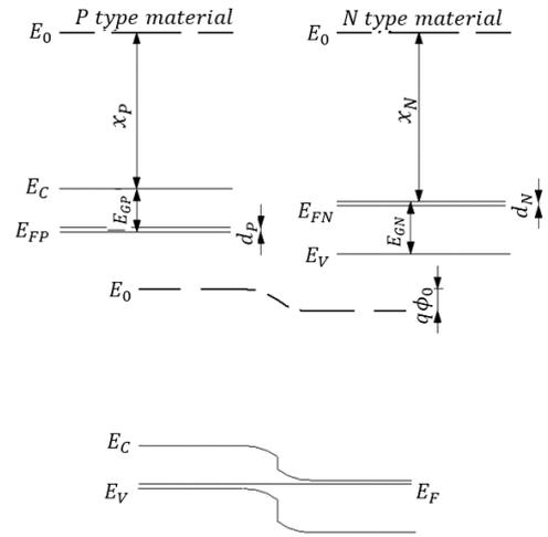
Fig. 3. General band diagram for a P-N heterojunctions.
