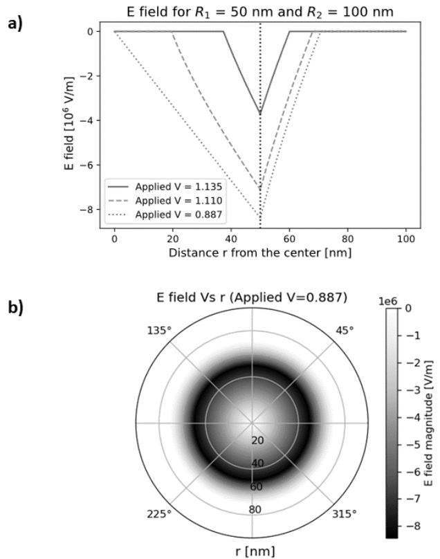
Fig. 11. a) Electric field in radial terms for the InP P-N homojunction. b) Top view of E in the InP P-N homojunction.
