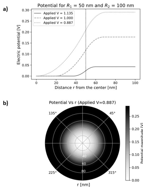
Fig. 12. a) Electric potential in radial terms for the P-N InP homojunction. b) Top view of the potential in the InP P-N homojunction.
