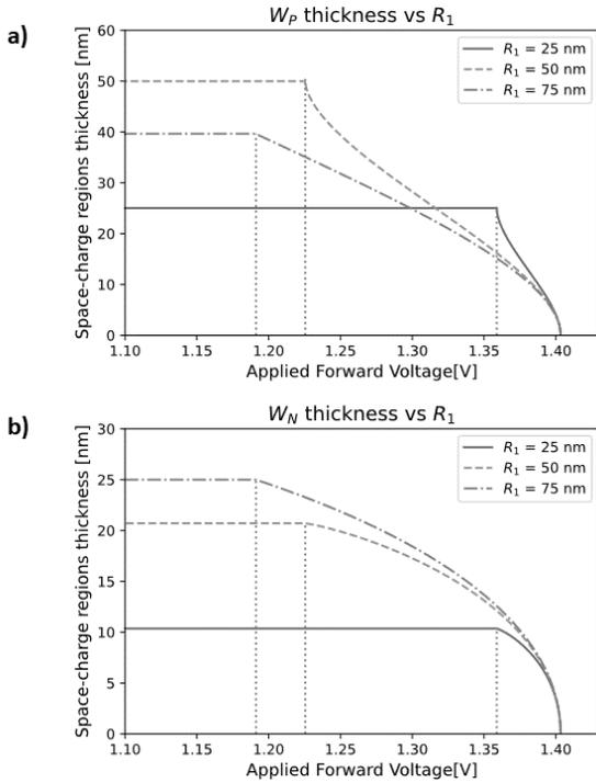
Fig. 8. a)  $w_P$  thickness as a function of the core radius. b)  $w_N$  thickness behavior as a function of the core radius, for three different  $R_1$  values with a fixed  $R_2$ .
