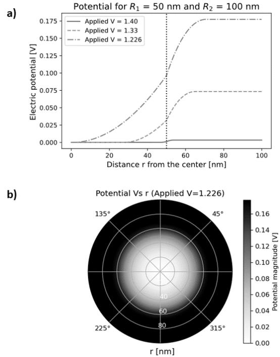
Fig. 7. a) Electric potential in radial terms for the P-N Heterojunction. b) Top view of the potential in the P-N Heterojunction.
