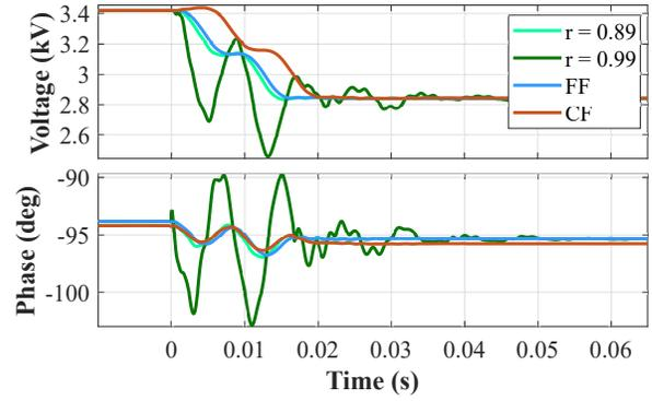
Fig. 5. Voltage's amplitude and phase angle results from the case study.
