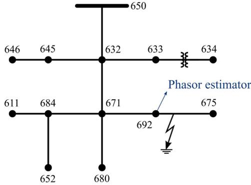
Fig. 4. IEEE 13 node test feeder one line diagram.
