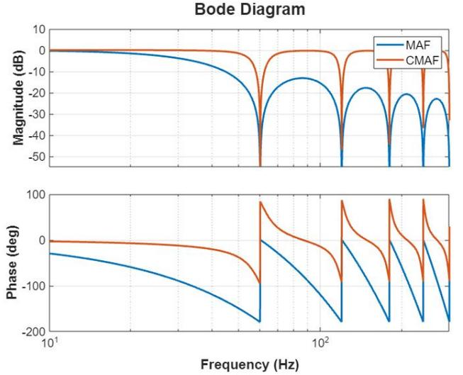
Fig. 1. Bode diagram of the MAF and the CMAF with  $r = 0.95$ .
