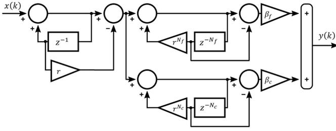
Fig. 2. Block diagram representation of the WCMAF.
