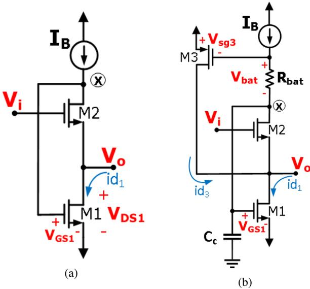
Fig. 1: a) Flipped Voltage Follower and b) Class AB Flipped Voltage Follower
