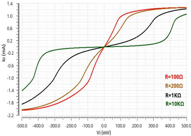
Fig. 3: DC transfer function characteristic
