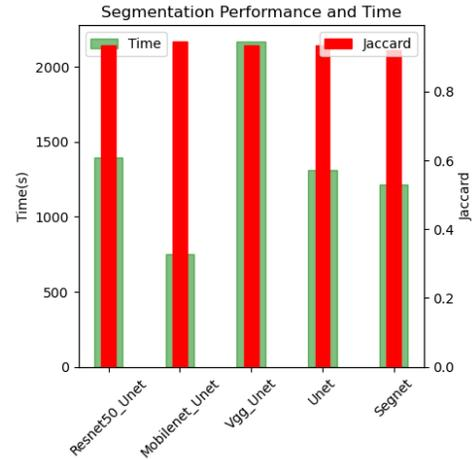
Fig. 1. Comparison of CNN models in terms of segmentation performance and time to train a CNN.
