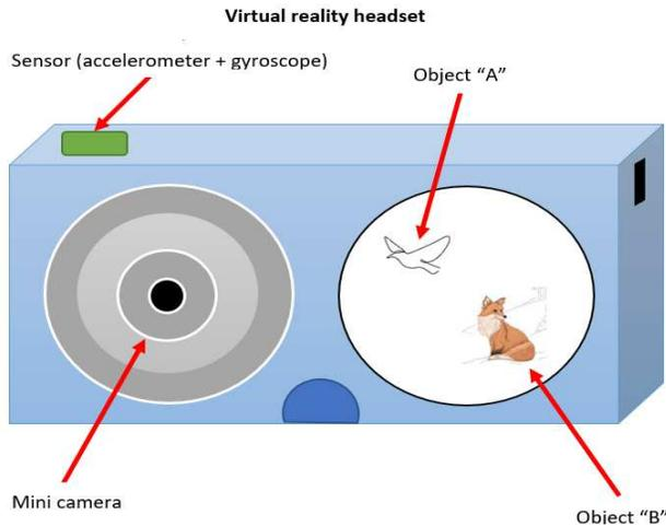
Fig. 1. Virtual reality headset and position of sensors for testing.
