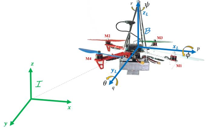
Fig. 1. Quadrotor in three-dimensional space
