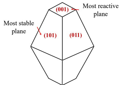
Fig. 3. The equilibrium shape of a  $\text{TiO}_2$  crystal in the anatase phase, according to the Wulff construction and surface energies calculated by Lazzeri *et al.* 2001. [34]
