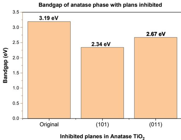
Fig. 4. Bandgap calculated in structures of Anatase TiO<sub>2</sub> with inhibited planes.
