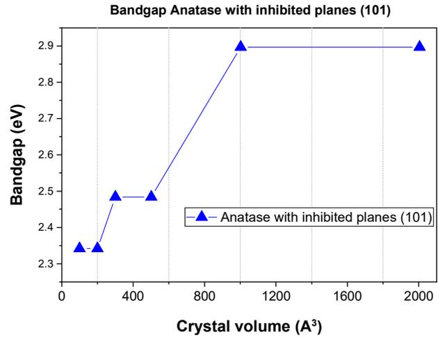
Fig. 5. Bandgap calculated for TiO<sub>2</sub> anatase structures with inhibited planes (101) and different crystal volumes
