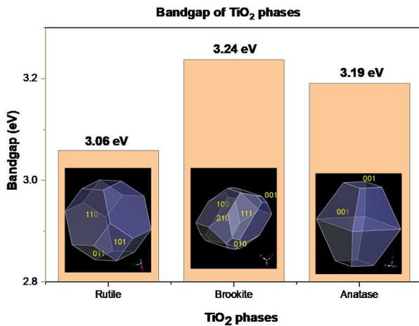
Fig. 2. Bandgap for the different phases of  $\text{TiO}_2$ .
