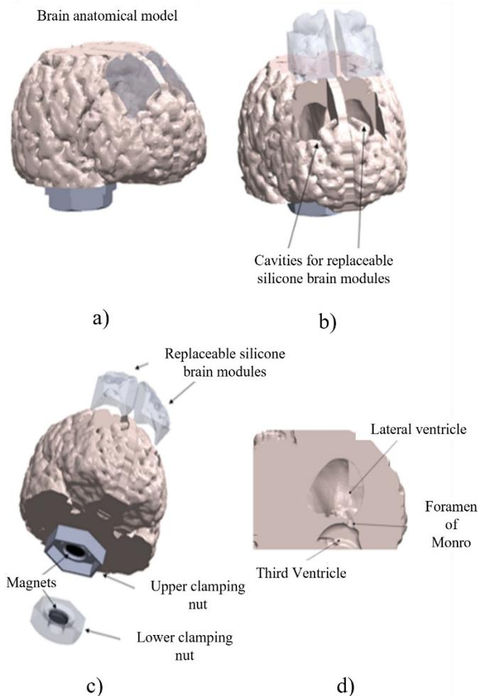
Fig. 4. Brain Model. a) Anatomical model of the full brain, b) placement of the replaceable silicone modules on the cavities, c) holding system of the brain model, d) Hollow ventricular system.
