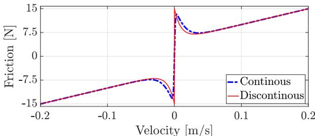
Fig. 3: Comparison of the continuous and discontinuous friction curves.
