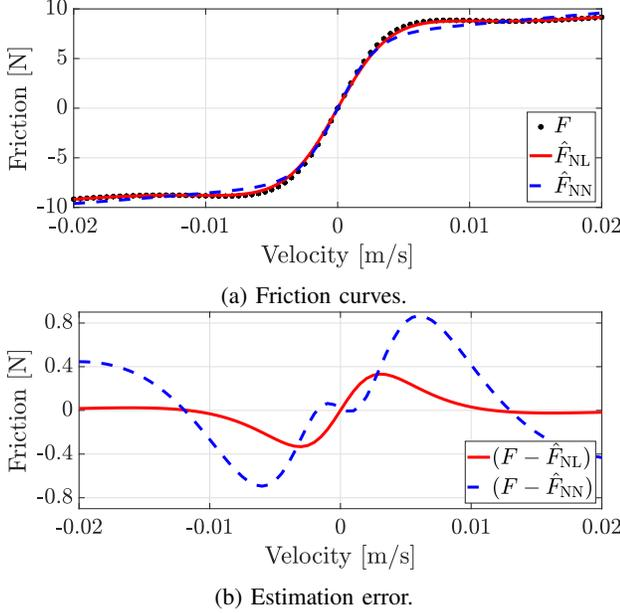
Fig. 5: Comparison of the estimated friction models.
