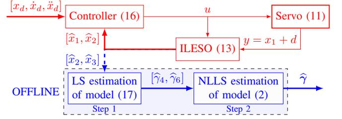
Fig. 2: Block diagram of the identification scheme.
