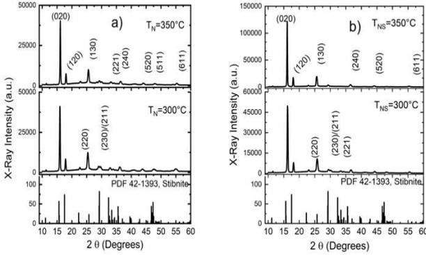
Fig. 1. XRD patterns annealed at 300 and 350°C in a) nitrogen and b) nitrogen-sulfur atmospheres.
