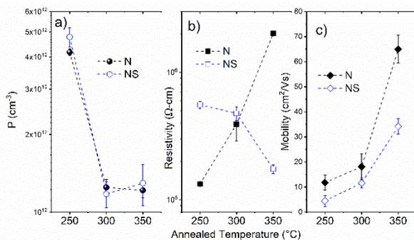
Fig. 4. Hall effect measurement of the samples annealed in nitrogen and nitrogen-sulfur atmospheres vs temperature a) hole concentration, b) resistivity and c) mobility.
