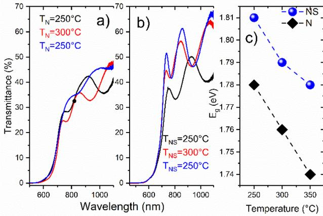
Fig. 3. Transmittance spectra of the samples annealed in a) nitrogen b) nitrogen-sulfur atmospheres, and c) bandgap of the thin films as a function of the annealing temperature.
