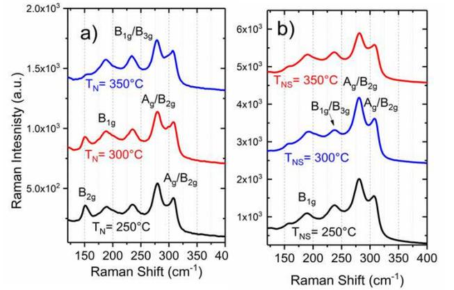
Fig. 2. Raman spectra of a) nitrogen and b) nitrogen-sulfur samples as a function of temperature.
