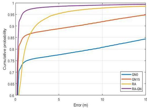
Fig. 5 Performance comparison of positioning methods in terms of CDF of the error.
