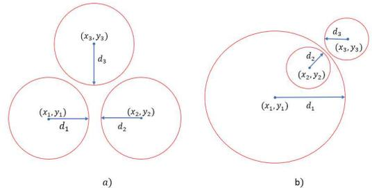
Fig. 2 Cases where there is no solution due to circles do not touch each other a) circles are in the exterior of each other b) one or two circles are inside the other one.
