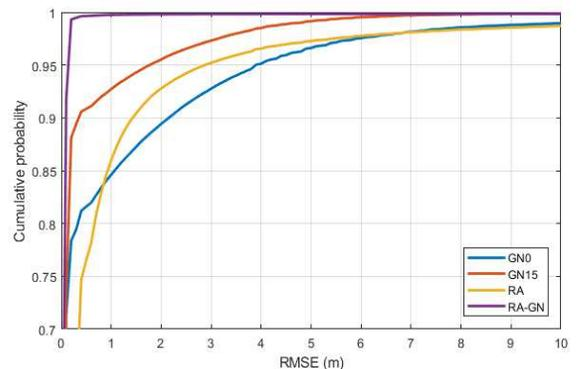
Fig. 4 Performance comparison of positioning methods in terms of CDF of the RMSE.
