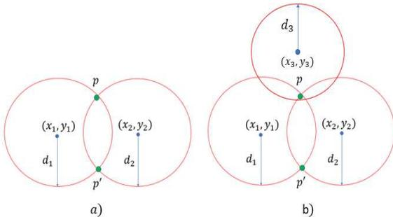
Fig. 1 Comparison of intersection points between circles a) ambiguity with two circles, b) solution by trilateration.
