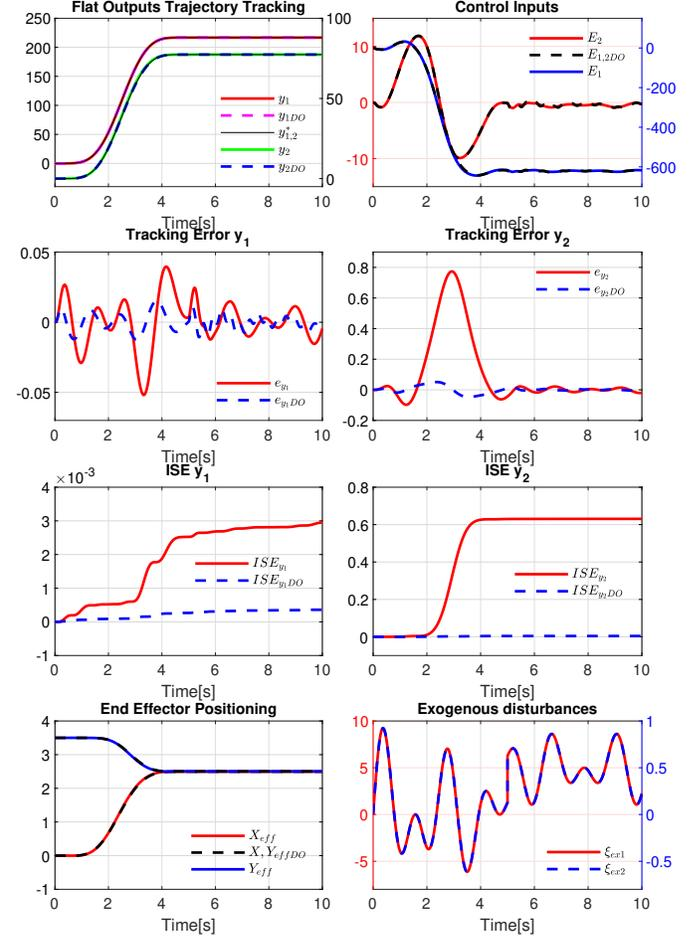
Fig. 4: Comparison between ROESO-ADRC and DOB+ADRC.
