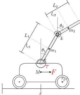
Fig. 3: The moving crane with flexibility.
