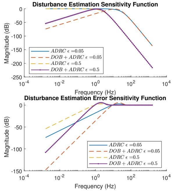
Fig. 2: Bode responses for representative transfer functions
