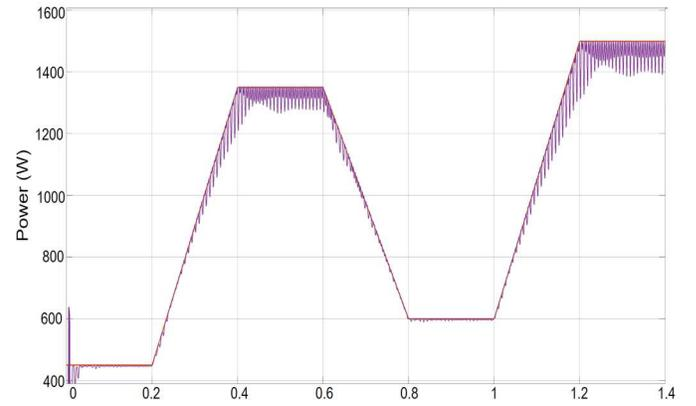
Fig. 7. Ideal power generated by the PV array and true power extracted for the multilevel inverter
