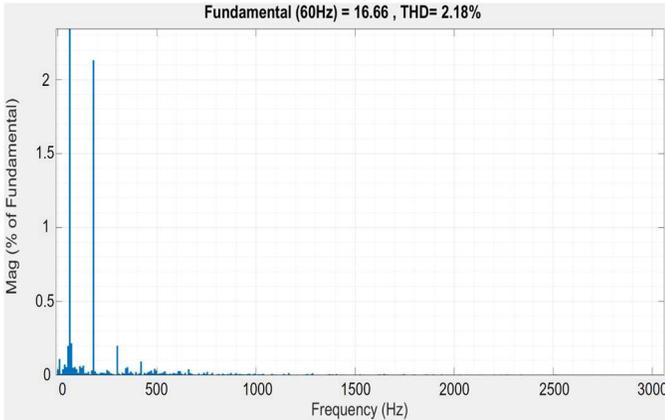
Fig. 10. THD of current with solar radiation of  $1000 \text{ W/m}^2$
