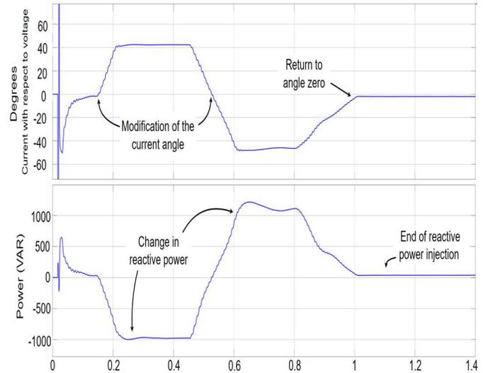
Fig. 11. The angle of the current concerning the voltage and reactive power injected into the grid
