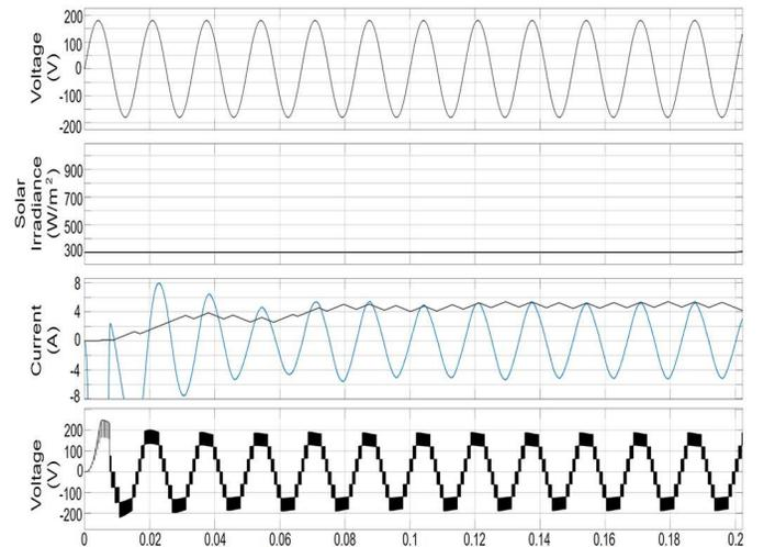
Fig. 8. Time instant at which the proposed control begins to synchronize with the single-phase voltage grid
