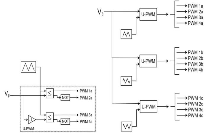
Fig.5. Scheme of the 7-level modulation technique
