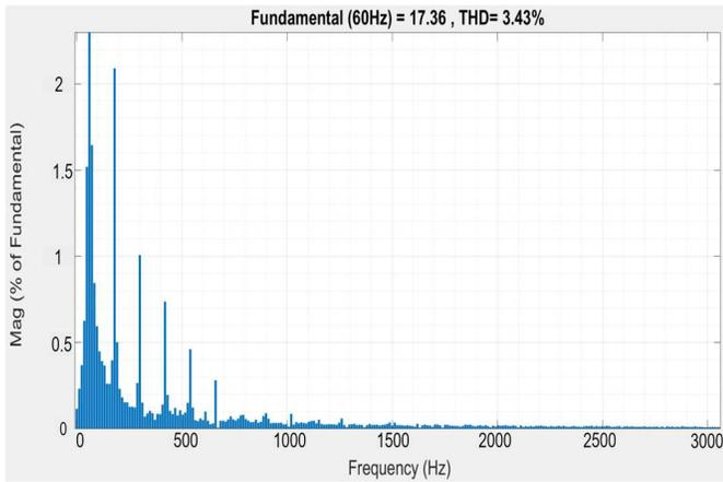
Fig.13. THD of the injected current when generating 1150 VAR of reactive power
