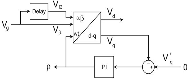
Fig.4. PLL block diagram
