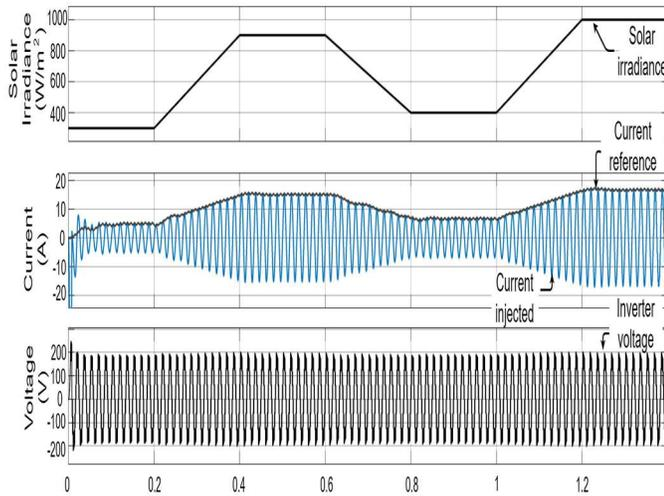
Fig. 6. Performance of the proposed control during peak current tracking with variable solar radiation.
