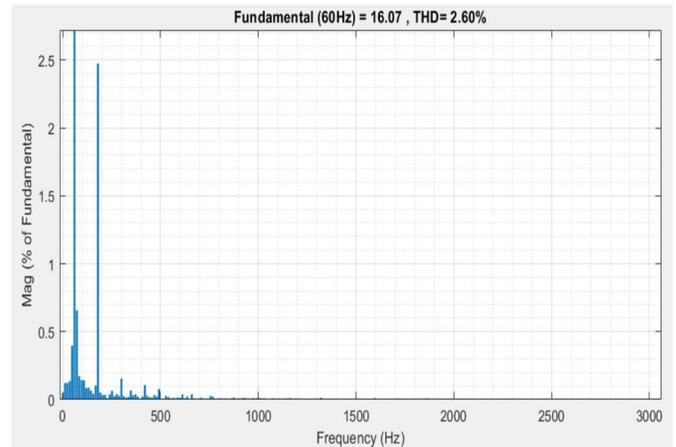
Fig.12. THD of the injected current when generating -975 VAR of reactive power
