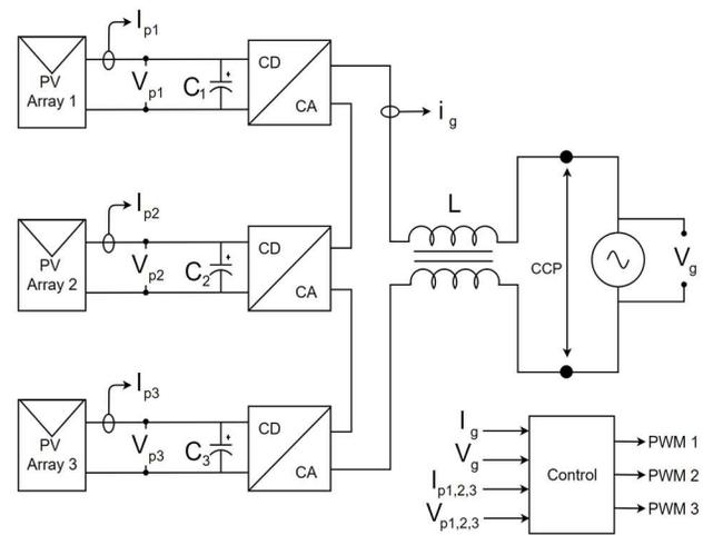
Fig. 1. Simplified diagram of the single-phase 7-level inverter based on three cascaded H-bridges.
