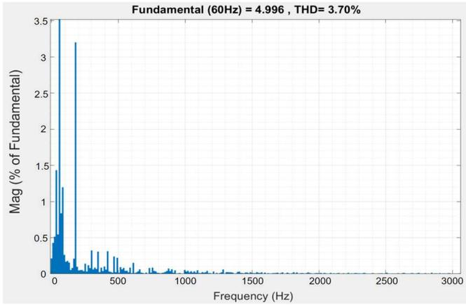
Fig. 9. THD of current with solar radiation of  $300 \text{ W/m}^2$
