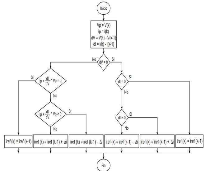
Fig. 3. Flowchart of the MPPT algorithm used for the calculation of the reference current.
