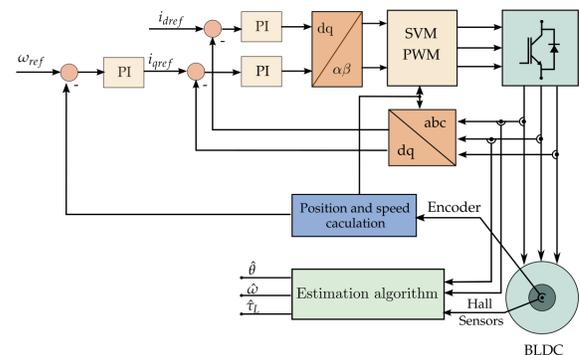
Fig. 1: Field oriented control and estimation algorithm.
