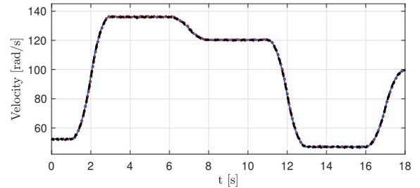
(a) Estimated velocity  $\hat{\omega}$  (---), estimated velocity by FAST  $\hat{\omega}_F$  (-.-) vs encoder velocity  $\omega_{enc}$  (—)
