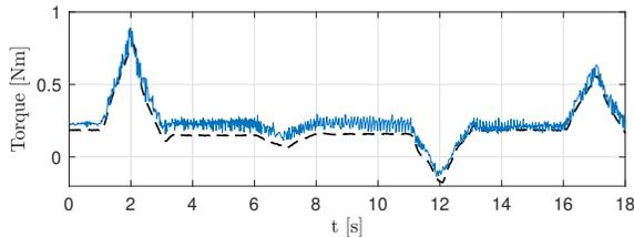
Fig. 7: Experimental results with flywheel: estimated load torque  $\hat{\tau}_L$  (---) vs estimated load torque by FAST  $\hat{\tau}_{LF}$  (—).
