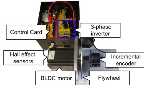
Fig. 2: Experimental platform.
