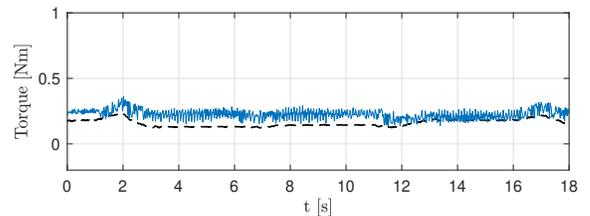
Fig. 5: Experimental results without load: estimated load torque  $\hat{\tau}_L$  (---) vs estimated load torque by FAST  $\hat{\tau}_{LF}$  (—).
