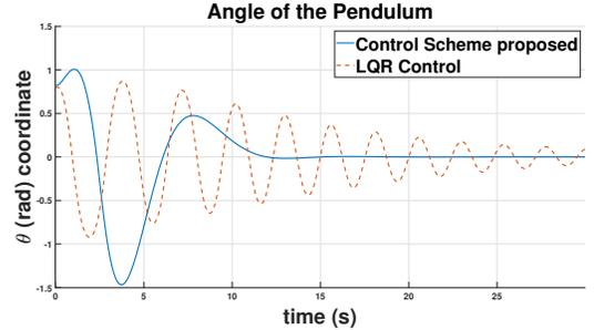
Fig. 4. Closed-loop response of the  $\theta$  coordinate.
