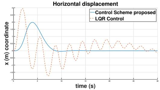
Fig. 3. Closed-loop response of the  $x$  coordinate.
