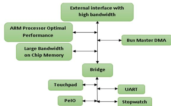
Fig 1. Typical system for ARM & AMBA
