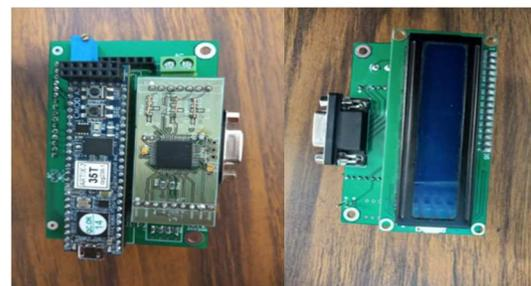
Fig. 8. Top and bottom view of the board implemented for the prototype.
