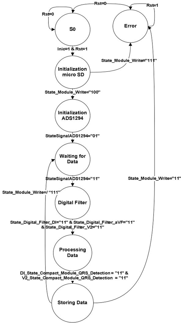
Fig. 2. General state machine implemented in FPGA.
