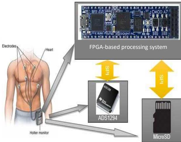
Fig. 1. Main components of the 3-channel ambulatory system.
