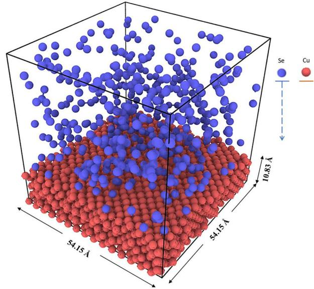
Figure 2. General process of the deposit of Se (blue) on the Cu (red) buffer layer.
