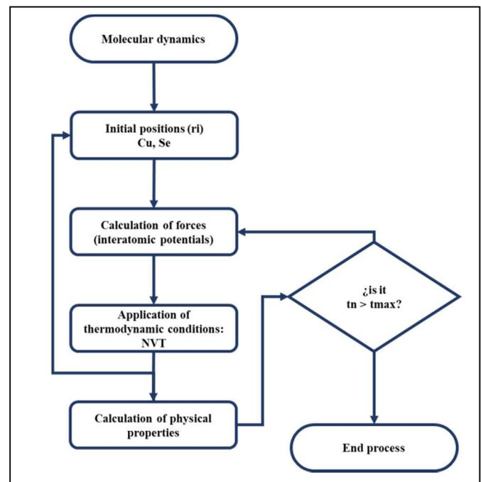
Figure 1. Computational flow diagram process.
