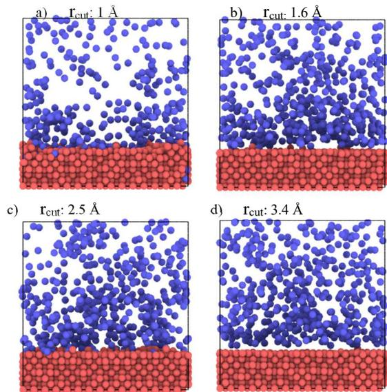
Figure 5. Se evaporation on Cu buffer layer at different  $r_{cut}$ , a) 1 Å, b) 1.6 Å, c) 2.5 Å and d) 3.4 Å. With 20 k time steps.
