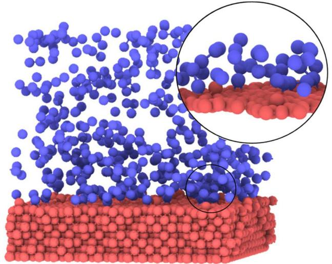
Figure 3. . Cu-Se interactions at surface. Velocity @550 K, cutoff:  $2.5 \text{ \AA}$ , 20k time steps. Blue and rose spheres represent Selenium and copper atoms respectively.
