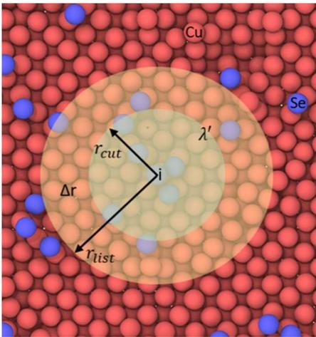
Figure 4. Representation of the cut off radius for Se atoms.
