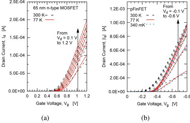
Fig. 2: Transfer characteristics for both, a) 65 nm n-type MOSFET and b) 14 nm p-type finFET from 300 K down to 77 K, with step of 0.1 V
