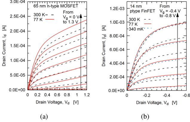
Fig. 1: Output characteristics for both, a) 65 nm n-type MOSFET and b) 14 nm p-type finFET from 300 K down to 77 K, with step of 0.1 V
