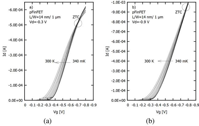
Fig. 7: ZTC comparative from 300 K to 340 mK with a)  $V_d = -0.3$  V, b)  $V_d = -0.9$  V.
