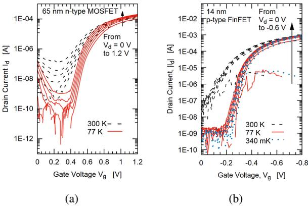
Fig. 3: Transfer characteristics for both, a) 65 nm n-type MOSFET and b) 14 nm p-type finFET from 300 K down to 77 K, in semi-log format, with step of 0.1 V
