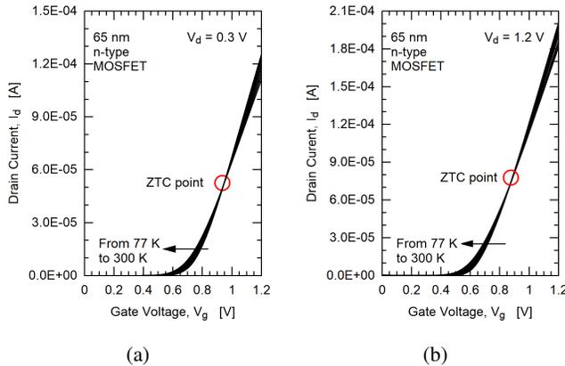
Fig. 8: ZTC comparative from 300 K to 77 K with a)  $V_d = 0.3$  V and b)  $V_d = 1.2$  V.
