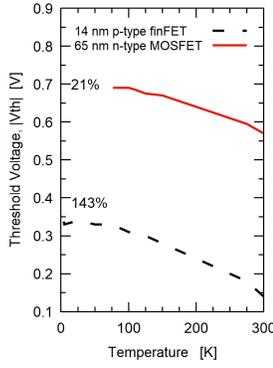
Fig. 4: Threshold Voltage  $V_{th}$  for both, 14 nm and 65 nm devices vs Temperature.
