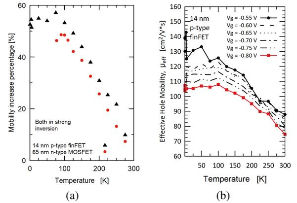
Fig. 6: a) Comparison of carrier mobility increase vs Temperature for the two devices, and b) hole mobility vs Temperature for the 14 nm finFET.
