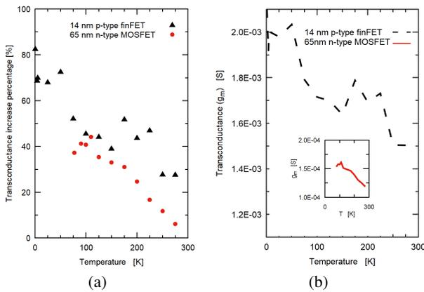
Fig. 5: Comparative of a) transconductance increase percentage and b) actual transconductance values for 65 nm and 14 nm devices.
