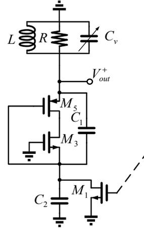
Fig. 3. The half circuit of the proposed oscillator
