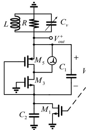
Fig. 4. Proposed the suitable half circuit to calculate  $\Gamma_{M_5}$
