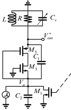
Fig. 5. The suitable half circuit to calculate  $\Gamma_{M1}$
