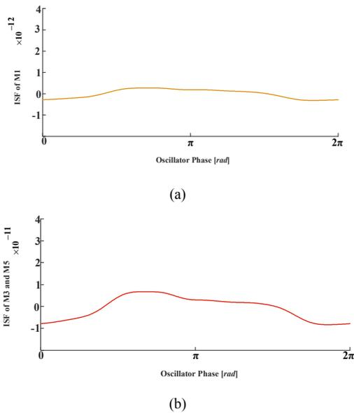
Fig. 6. The simulated ISFs of (a) M1 (b) M3 and M5 for thermal noise
