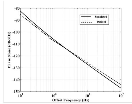
Fig. 7. The simulated and derived phase noise
