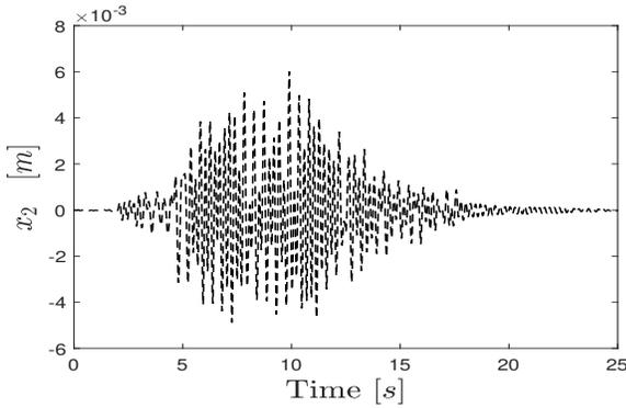
Fig. 4: Uncontrolled building response subject to 1985 earthquake excitation
