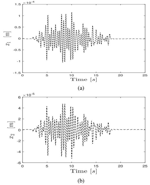
Fig. 7: System response with  $\mathcal{H}_\infty$  controller under 1985 earthquake excitation (a)  $x_1$  (b)  $x_2$
