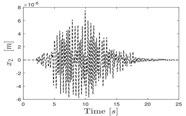
Fig. 6: Displacement of second floor with  $\mathcal{H}_\infty$  controller under 1985 earthquake excitation
