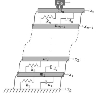
Fig. 1: Building with controller in the  $n$ -floor
