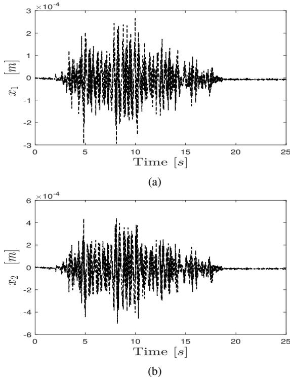
Fig. 8: System response with PD controller for 1985 earthquake excitation (a)  $x_1$  (b)  $x_2$
