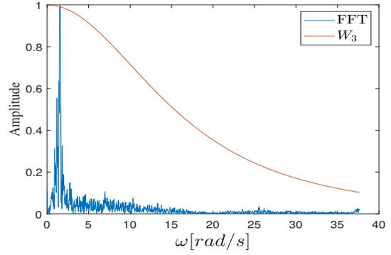
Fig. 3: FFT of 1985 earthquake data vs Weighted function  $W_3$
