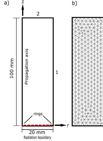
Fig. 1. (a) FEM geometry. (b) representation of the triangular mesh used (not showing the actual size).
