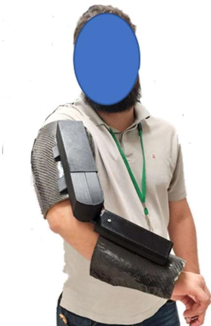
Fig. 6. Developed elbow exoskeleton.
