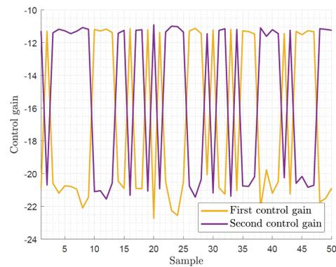
Fig. 6. Oscillation of the convergence values for control gains, with the presence of local minimus.
