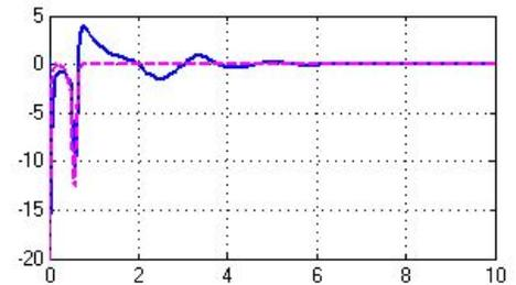
Fig. 4. Attitude first derivative  $\dot{\theta}$  in continuous line and attitude desired  $\dot{\theta}_d$  first derivative in dashed line. The vertical axis corresponds to the PVTOL attitude orientation angle first derivative (rad/s) and the horizontal axis corresponds to the time ( $t$ ) in seconds.
