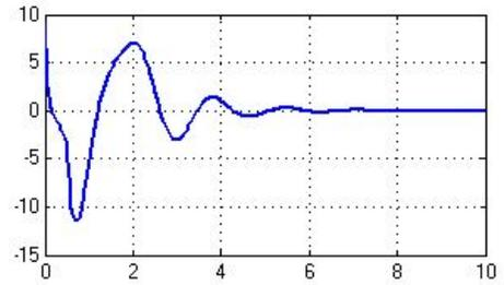
Fig. 11. Horizontal displacement second derivative  $\ddot{x}$ . The vertical axis corresponds to the PVTOL horizontal displacement second derivative  $\ddot{x}$  ( $m/s^2$ ) and the horizontal axis corresponds to the time ( $t$ ) in seconds.
