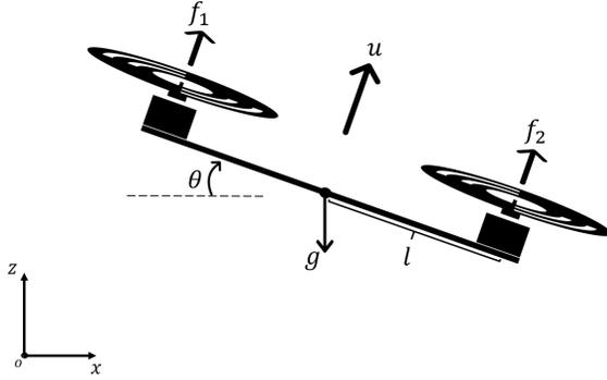
Fig. 1. PVTOL diagram. Where  $f_1$  and  $f_2$  are the control forces,  $l$  is the distance,  $m$  is the mass,  $\theta$  is the angle of the aircraft with respect to the horizontal line,  $g$  is the gravitational acceleration,  $x$  is the horizontal displacement and  $z$  is the vertical displacement.
