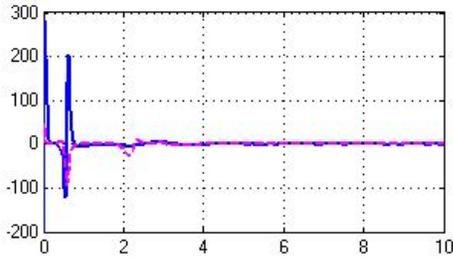
Fig. 5. Attitude second derivative  $\ddot{\theta}$  in continuous line and attitude desired  $\ddot{\theta}_d$  second derivative in dashed line. The vertical axis corresponds to the PVTOL attitude orientation first derivative ( $rad/s^2$ ) and the horizontal axis corresponds to the time ( $t$ ) in seconds.
