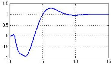
Fig. 6. Altitude  $z$ . The vertical axis corresponds to the PVTOL altitude  $z$  in meters ( $m$ ) and the horizontal axis corresponds to the time ( $t$ ) in seconds.
