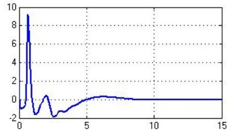
Fig. 12. Control input  $u$ . The vertical axis corresponds to the PVTOL control input  $u$  in newtons ( $N$ ) and the horizontal axis corresponds to the time ( $t$ ) in seconds.
