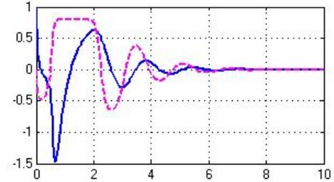
Fig. 3. Attitude  $\theta$  in continuous line and attitude desired  $\theta_d$  in dashed line. The vertical axis corresponds to the PVTOL attitude orientation angle (rad) and the horizontal axis corresponds to the time ( $t$ ) in seconds.
