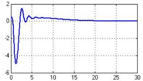
Fig. 10. Horizontal displacement first derivative  $\dot{x}$ . The vertical axis corresponds to the PVTOL horizontal displacement first derivative  $\dot{x}$  ( $m/s$ ) and the horizontal axis corresponds to the time ( $t$ ) in seconds.
