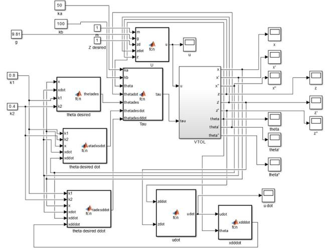
Fig. 2. Simulink diagram. The blocks that contain:  $\theta$  values and their derivatives (calculated in the previous section), PVTOL model (corresponding to section 2), values of selected gains and the input control  $u$  and its derivative.
