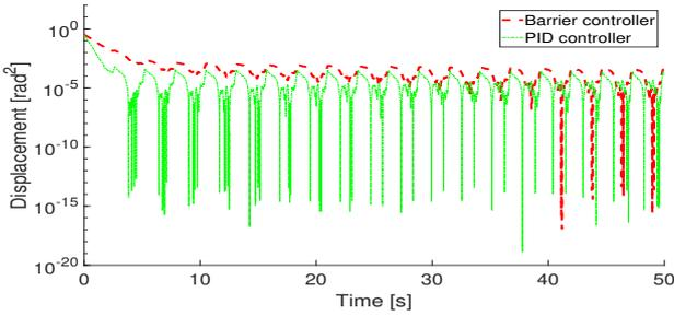
Fig. 7. Logarithmic comparison of the error norm signal between the proposed and the PID controllers for the hip articulation.
