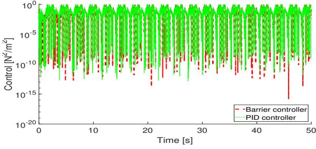
Fig. 6. Logarithmic comparison of the control norm signal between the proposed and the PID controllers for the knee articulation.
