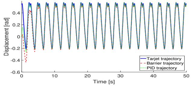
Fig. 3. Comparison of trajectory tracking performance between the proposed and PID controllers at the hip joint in the biped robot
