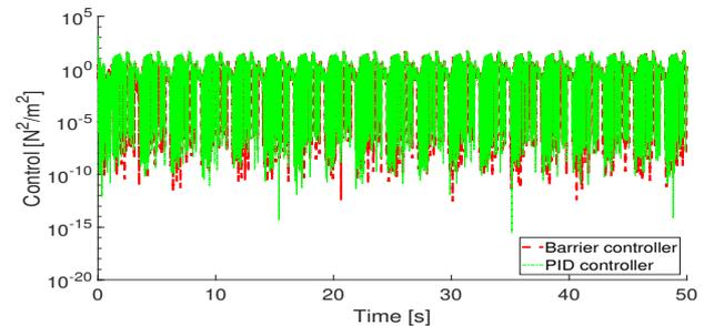
Fig. 5. Logarithmic comparison of the control norm signal between the proposed and the PID controllers for the hip articulation.
