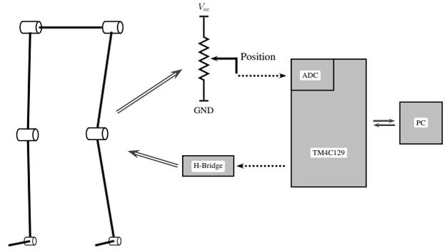
Fig. 2. Electronic instrumentation arrangement
