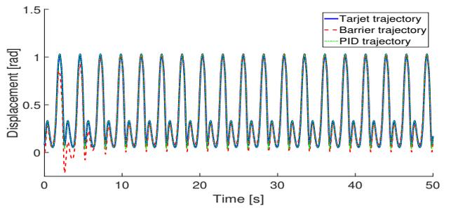
Fig. 4. Comparison of trajectory tracking performance between the proposed and PID controllers at the knee joint in the biped robot
