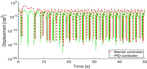
Fig. 8. Logarithmic comparison of the error norm signal between the proposed and the PID controllers for the knee articulation.
