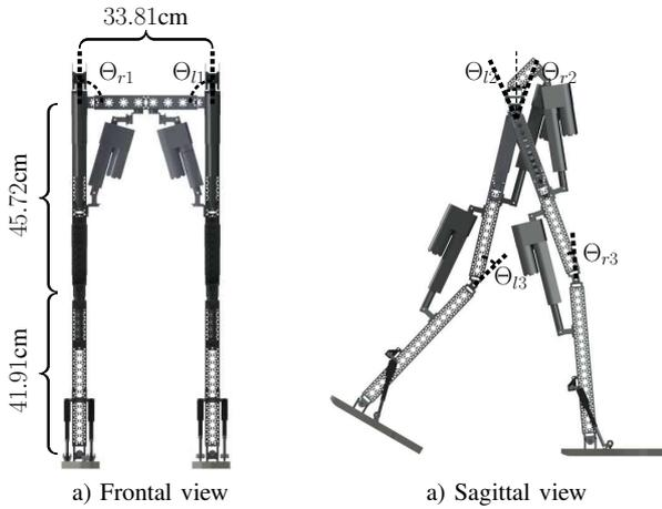
Fig. 1. Dimensions and degrees of freedom considered in the structure of the biped robot
