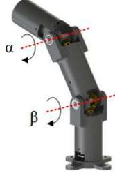
Fig. 2. Two-link manipulator
