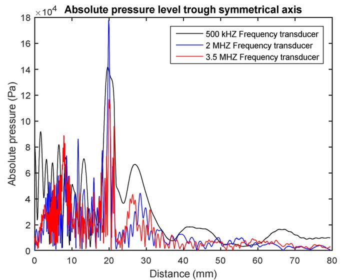
Fig. 3 – Pressure distribution along the symmetric axis of the model. It was made a parametric swept to obtain these results. The black line represents the result of 500 kHz, the blue line is the 2 MHz and the red line is the 3.5 MHz.
