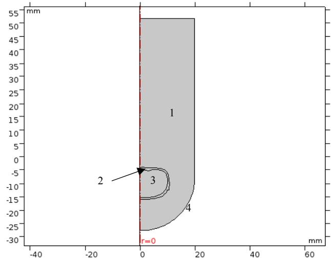
Fig. 1 – Geometry of the simulation. Every domain is different: 1.- Water, 2.- Skull bone, 3.- Brain tissue. Boundary 4 represents the transducer.
